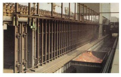
Figure 1: "Coke Side" of a By-Product Coke Oven Battery. The oven has just been "pushed" and railroad car is full of incandescent coke that will now be taken to the "quench station".
